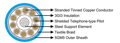
**Conductors:** Flexible stranded tinned copper conductor, class 5 according to DIN VDE 0295. **Insulation:** EPR type 3GI3.
